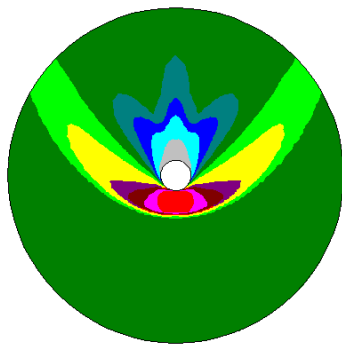
Cross sectional density contour for Mach 1.8 flow past a 5° cone at 45° angle of attack.
